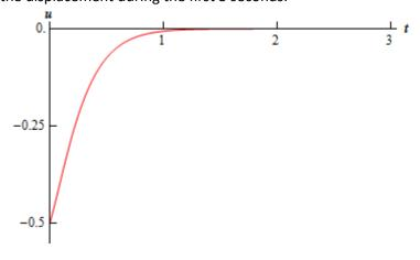
Notice that the "vibration" in the system is not really a true vibration as we tend to think of them. In the critical damping case there isn't going to be a real oscillation about the equilibrium point that we tend to associate with vibrations. The damping in this system is strong enough to force the "vibration" to die out before it ever really gets a chance to do much in the way of oscillation.
