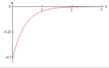
Notice an interesting thing here about the displacement here. Even though we are "over" damped in this case, it actually takes longer for the vibration to die out than in the critical damping case. Sometimes this happens, although it will not always be the case that over damping will allow the vibration to continue longer than the critical damping case.
