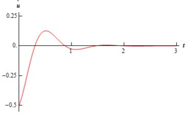
In this case we finally got what we usually consider to be a true vibration. In fact, that is the point of critical damping. As we increase the damping coefficient, the critical damping coefficient will be the first one in which a true oscillation in the displacement will not occur. For all values of the damping coefficient larger than this (*i.e.* over damping) we will also not see a true oscillation in the displacement.
