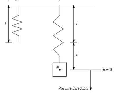
As denoted in the sketch we are going to assume that all forces, velocities, and displacements in the downward direction will be positive. All forces, velocities, and displacements in the upward direction will be negative.
